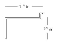
Rite Strips are L shaped PVC extrusions used to minimize the large radius on the top of a fiberglass pool for the use of a cantilever form.
